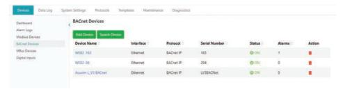
**NOTE:** After adding a new device to the gateway it may take up to 3-4 minutes for the status to show 'ON'. If after 3-4 minutes the device is showing an 'OFF' status, double-check the configuration settings to ensure everything is set correctly.
