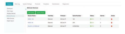
**NOTE:** After adding a new device to the gateway it may take up to 3-4 minutes for the status to show 'ON'. If after 3-4 minutes the device is showing an 'OFF' status, double-check the configuration settings to ensure everything is set correctly.
