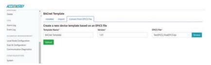
Once the name, version and EPICS file has been uploaded users can click on *Upload*. Users will be able to configure and specify which parameter they want to include in the BACnet template, once the parameters are configured click on *Save* at the bottom of the page.
