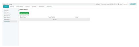
Users will be required to enter a Device name for the virtual device. Once the name is selected for the device click on *Add Virtual Parameter* to start creating and adding the virtual parameters.
