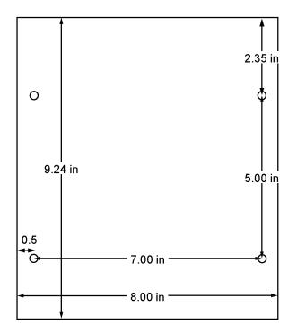
The AcquiSuite has 4 mounting holes for use with a #6 or #8 screw. The drawing above shows the relative position of the mounting holes.
