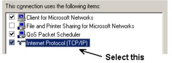
Note: If you have multiple ethernet cards, you may have multiple lines labeled "TCP/IP --> ethernet card". Locate the ethernet card that corresponds to the physical connection to the AcquiSuite and then select the TCP/IP option that is linked with that ethernet card.
